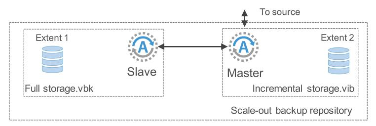
With SMB or DDBoost with automatic gateway server, master data mover is the source proxy.
